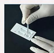
4. Suck the ground hair solution with a test tube, drop 3-5 drops into the hair detection plate, and observe the changes of the detection plate.
